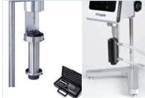
Small sample adapter for L, R and H viscometers.
