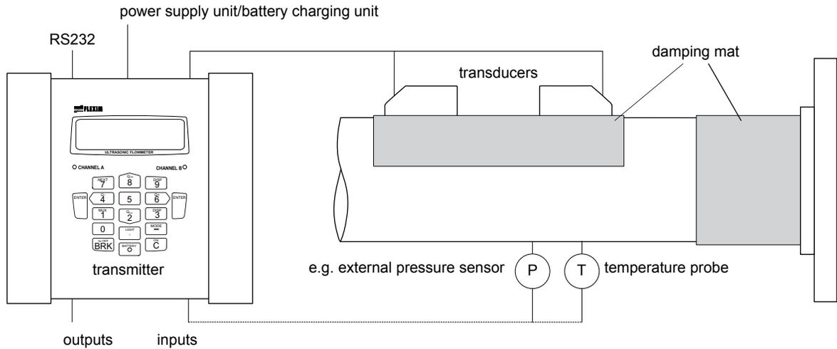
Example of a reflect arrangement with connection of the inputs to an external process pressure and process temperature measurement for standard volumetric flow rate calculation
